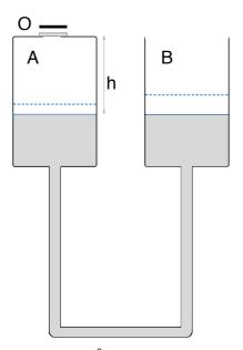
Two tanks of equal cross section of 100 cm<sup>2</sup> are connected by a tube as shown. Initially A is open to the atmosphere and water in both tanks is at the same level. The hole O is then closed and water is added in tank B until the level in the tank  $B = \frac{h}{2}$ .
