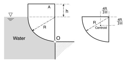
The uniform body A shown in the figure below has width b normal to the plane of the figure, and is in static equilibrium when pivoted about hinge O.The adjacent water is exerting a force on the body that is maintaining it in equilibrium. What is the density of this body if :
