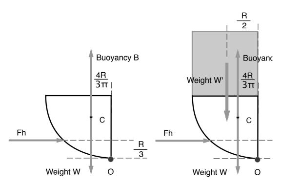
Free body diagram left figure with h = 0, all forces are shown except for the reaction at O since it produces no moment.
